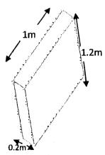
Fig 4.22: Volume of concrete required per metre length of wall
