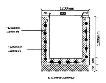
Fig. 4.25: Typical drain section with steel reinforcement and concrete
