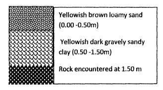
Fig 4.5: Soil profile loggings of naturally occurring soil layers in the project site
