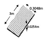
Fig 4.20: Size of wood for formwork
