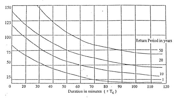
Figure 2.1 Graphs of Return Period, Intensity and Duration (which =T<sub>c</sub>)
