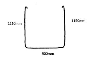
Fig. 4.26: Shape and dimension of wall and base bar
