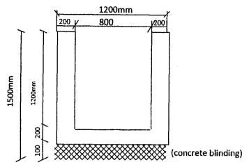
Fig. 4.17: Typical designed drain section
