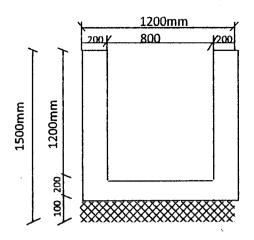
Fig. 4. 24: Typical drain section
