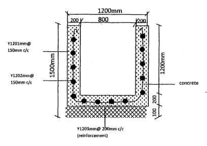
Fig.4.18: Typical designed drain section with reinforced concrete
