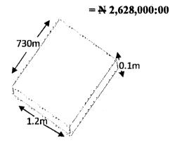
Fig 4.21: Volume of concrete required for blinding
