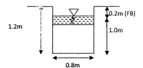
Fig. 3.3: Designed drain with freeboard
