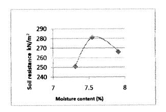
Fig. 4.12: Soil resistance characteristics charts of gully area
