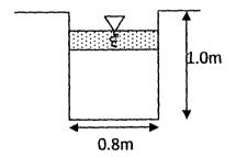
Fig. 3.2: Designed drainage channel
