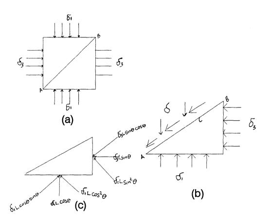
(a,b)--Stress acting on cubical unit in a granular mass
