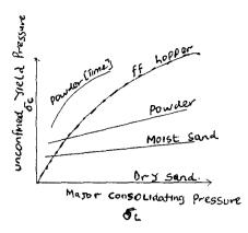
Fig.1.8: Critical flow factor FF of a hopper superimposed on flow function several solids (Jenike and Johnson Inc)
