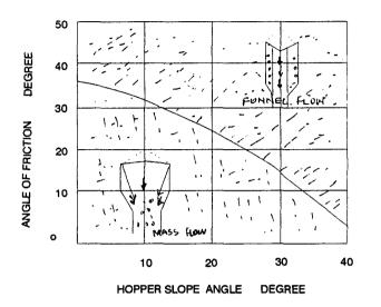
Fig.1.7- types of flow as affected by hopper slope angle and friction angle of solid hopper wall (Jenike and Johnson inc).
