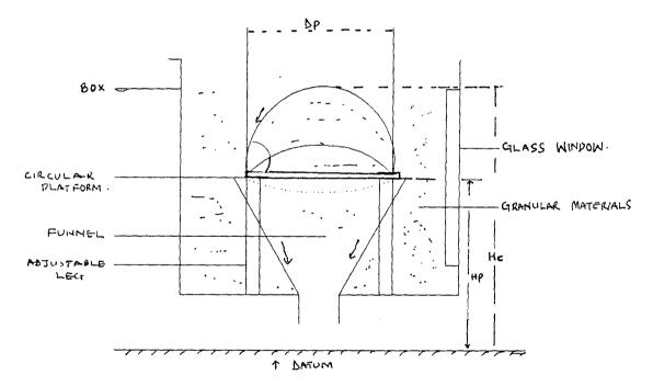
Fig. 1.1 - Fowler and Wyatt apparatus for measuring angle of repose of granular solid.
