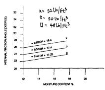
Fig.1.6b Variation of internal angle of friction with moisture content and density[Stewart, 1960].
