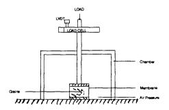
fig 1.5:Schematic for application of Triaxial compression test of agricultural grains.
