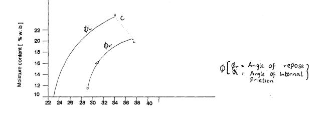
Fig 1.4:Variation of angle of repose and angle of internal friction with moisture content(Lorenzen, 1957).
