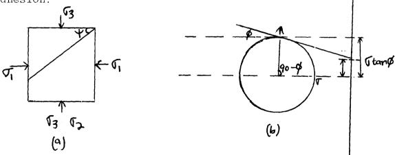
Fig. 1: Mohr-Coulomb Failure diagram
