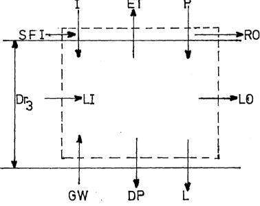
Fig. 2.3 Definition sketch for equation 2.3 Where, I irrigation (cm) = Ρ precipitation (rain) (cm)= SFI surface flow into the control volume (cm) subsurface lateral flow into the control volume (cm)  $\mathbf{LI}$ = groundwater seepage into the control volume (cm) GW =
