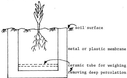
Fig. 2.3.2 A weighing lysimeter.
