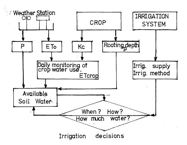
Fig. 1.0 Schematic representation of an irrigation management system. 1.6.3 Crop water requirement determination.
