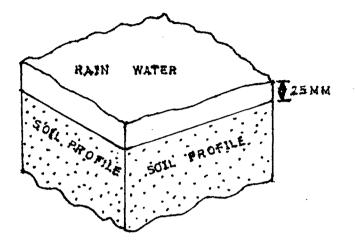
Fig. 3.6 Illustration of the depth of rainfall.
