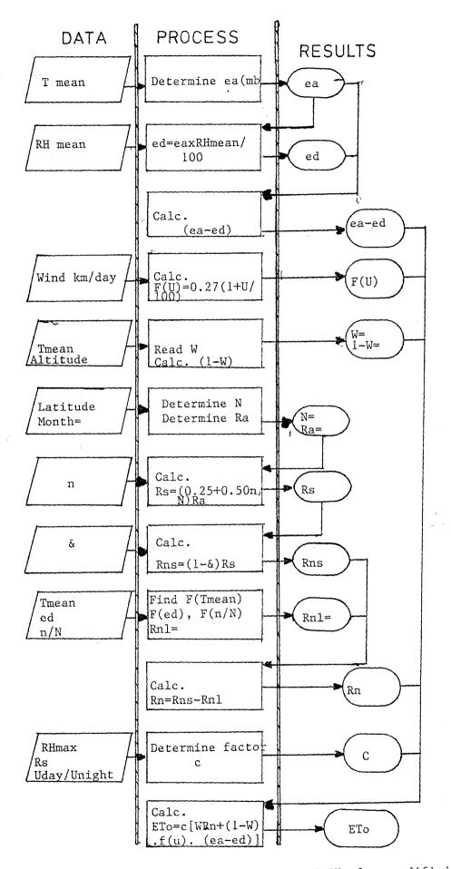
Fig. 4.8: Flow chart for determination of ETo from modified penman method.
