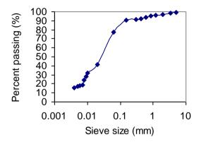
Fig.1. Particle size distribution for the natural soil.
