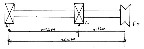
Fig I load on bearing
