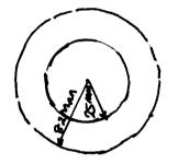
The volume of the metal sheet closure;  $Vmc = \pi (D^2 - d^2) \times t$   $-\frac{\pi}{4}$  D = 82mm d = 25mm t = 2.526mm  $\pi (D^2 - d^2) \times t$   $-\frac{\pi}{4}$
