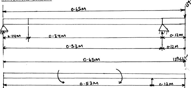
To determine the reaction RA and RC of the horizontal component.
