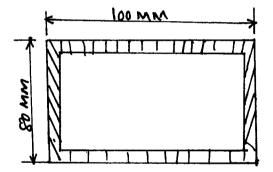
Length of outer portion Lo = 102.438mm Width of outer portion Bo = 82.438mm Length of internal portion Li = 100mm Width of internal portion Bi = 80mm
