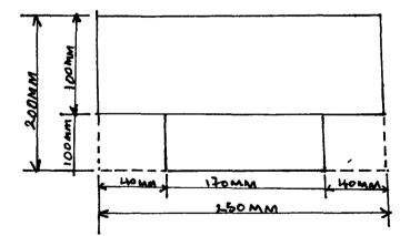
Weight of the entire mild steel sheet of guage 12, where the thickness is determine to be 2.526mm.
