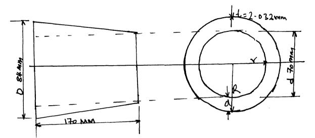
The use of gauge 16 metal mild sheet which has a thickness of 2.032m.
