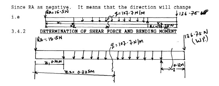
However, the shear force and bending moment can be determines as follows:-
