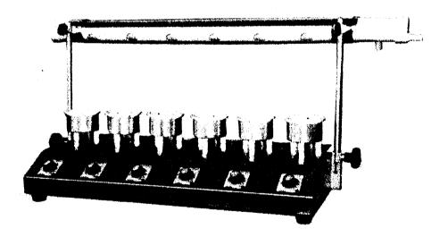
Plate 3.5: Micro Kjeldahl Digestion Unit
