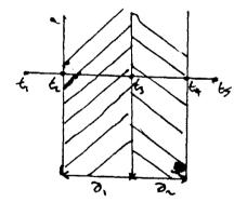
$q = \alpha a(t_1-t_2)$  ----- [1] Convection
