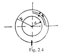
Considered the above figure an elemental cylinder within the cylinder at radius r and thickness dr.
