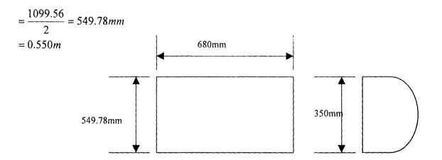
Now, the material volume of the water trough V<sub>vdw</sub> using a galvanized sheet of 16 gauge
