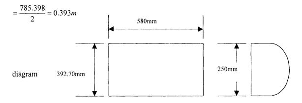
Now, the material volume of the rotary perforated cylinder  $V_{TR}$ ; using a galzvanized sheet hauge 16
