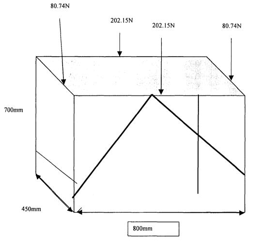
Fig 3.2 Load Distribution on The Frame
