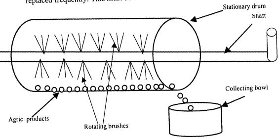
brushes are made of fibre, rubber, sponge or other material and may have to be replaced frequently. This must be considered in evaluating this type of washer.
