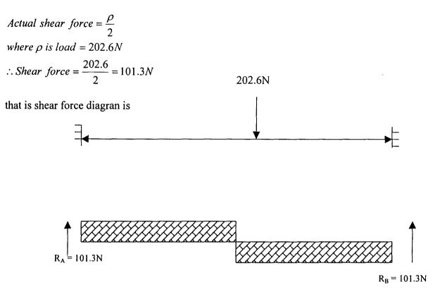
Actual shear stress =  $\frac{Shear force}{Area of section}$ where Area of section =  $3.08cm^2$  (from the steel designers' manual table)  $\therefore$  Actual shear stress =  $\frac{101.3}{3.08 \times 10^2} = 0.33N / mm$ sin ce 0.33N / mm is less than 100N / mm hence the section is okay
