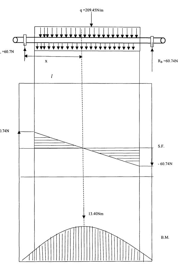
Fig 3.1The Shear Force And Bending Moment Diagram
