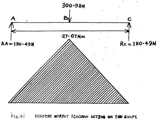
BENDING NOMENT DIAGRAM ACTING ON THE SHAFT,
