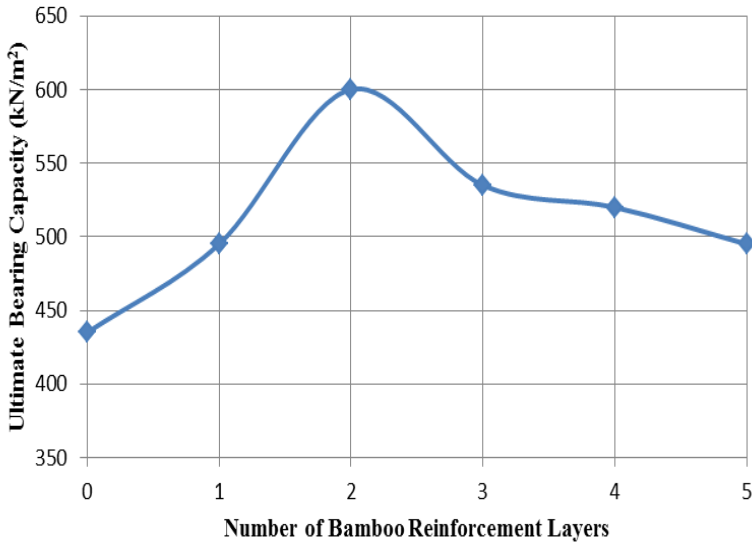
Figure 7: Variation of ultimate bearing capacity with increase in number of reinforcement layers
