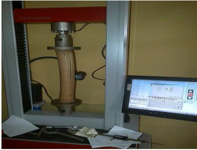
Figure 1: Bamboo culm in compression
