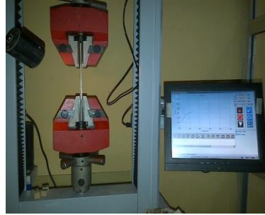
Figure 2: Bamboo splint in tension
