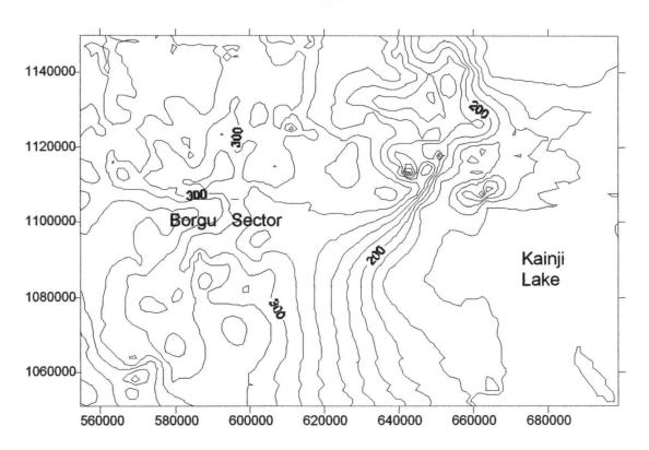
Fig.4.7: Contour map generated from 600 spots height extracted from topomaps
