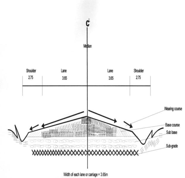
Fig. 4.2 Geometry of Zuba – Gwagwalada carriageway
