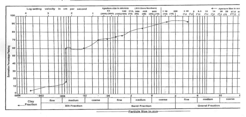
Fig. 4.9: Particle Size Distribution of 'control' cross section
