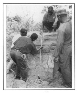
Plate xvii Insitu Borelog within Failed Carriageway Section Source: Author's field work Zuba -Gwagwalada 2007
