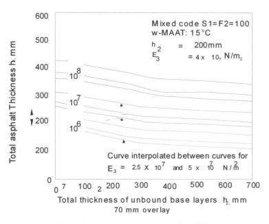
Fig. 2.2 Determination of Overlay Thickness
