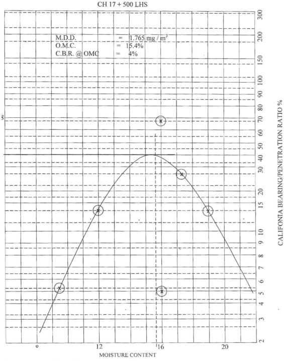
Fig. 4.11: Compaction Test of 'Control' cross section Source: Author's Fieldwork, 2007
