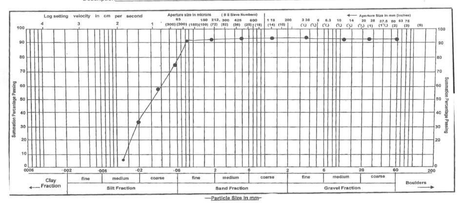
Fig. 4.6: Particle Size Distribution of Failed cross section Source: Author's fieldwork, 2007
