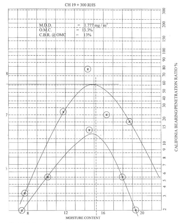
Fig. 4.12: California Bearing Ratio of 'Control cross section Source; Author's fieldwork, 2007
