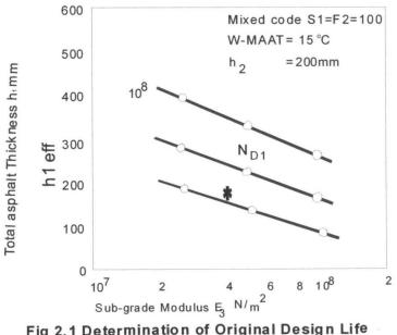
Fig 2.1 Determination of Original Design Life
