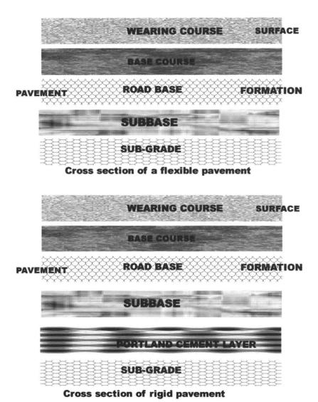
Fig. 1.3 Typical Flexible and Rigid Pavements
