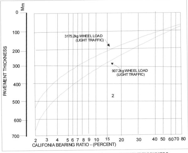
**Fig2.4:** SPECIFIC CBR VALUES PER PAVEMENT THICKNESS. Source: Air Field Pavement Development and Design Department, USA (1999)
