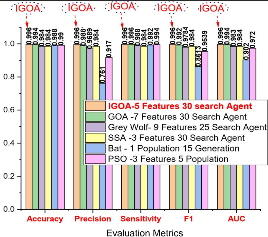
**Figure 4.200: Performance Evaluation of the Various Algorithm Used**
