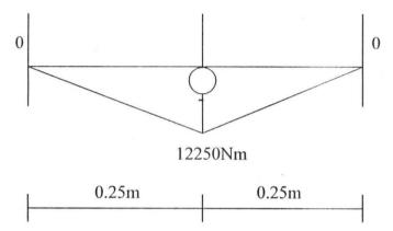
Fig. 3.2 Bending moment diagram
