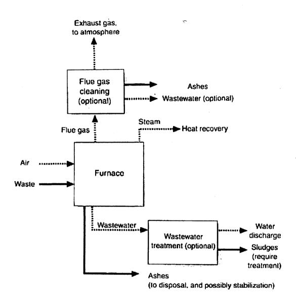
Figure 2.5. Simplified flow scheme of incinerator
