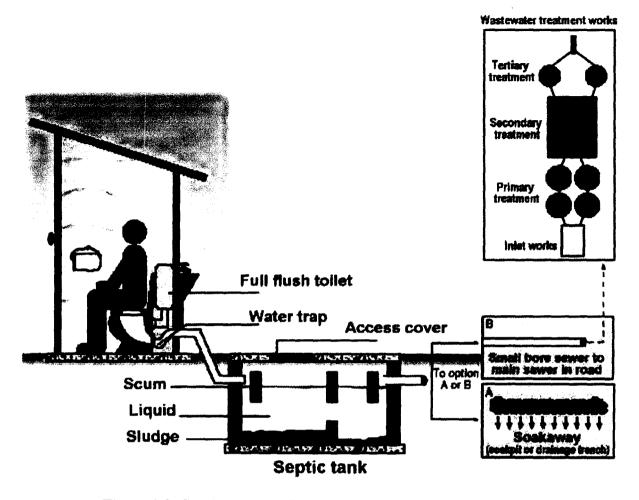
Figure 2.2: Septic Tank and Soakaway or Small Bore Solid-Free Sewer
