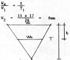
Fig. 3.4 Bottom width of V-belt
