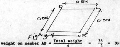
Assuming that the load  $W_{AB}$  is uniformly distributed so that the reaction at A and B is given by
