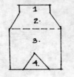
Volume of 1st cylinder =  $\pi r^2 h$   $\pi (0.1)^2 \times 0.015 = 0.00047m^3$ Volume of frustrum of cone 2 = volume of large cone - volume of small cone Volume of large cone =  $1/3 \pi r_1 H$ =  $1/3 \pi (0.1) \times 0.06 = 0.006m$
