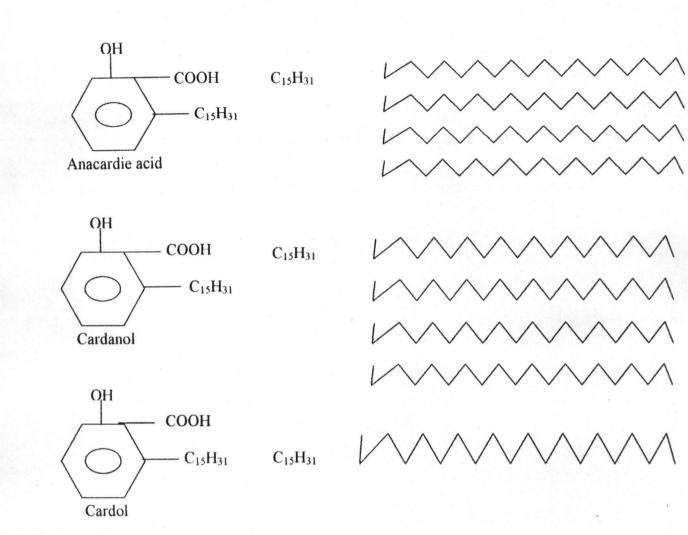
In technical (i.e heat extracted) CNSL, heating process leads to decarbonxylation of the anacardic acid to form cardonol. Typically, the composition of technical CNSL is 52% cardonol. 10% cardol 30% polymeric material, with the remainder being made up of other substances.
