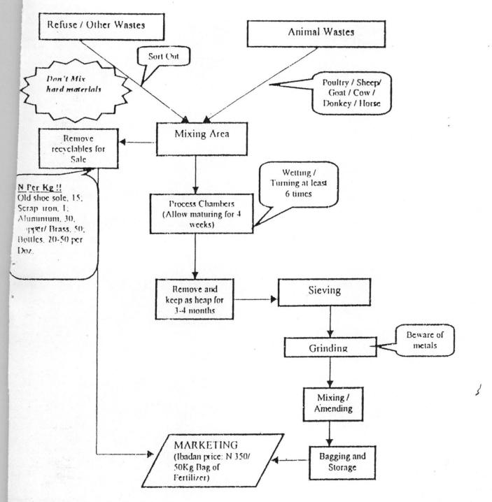
Figure 1: Flow sheet for the processing of wastes into organic fertilizer.
