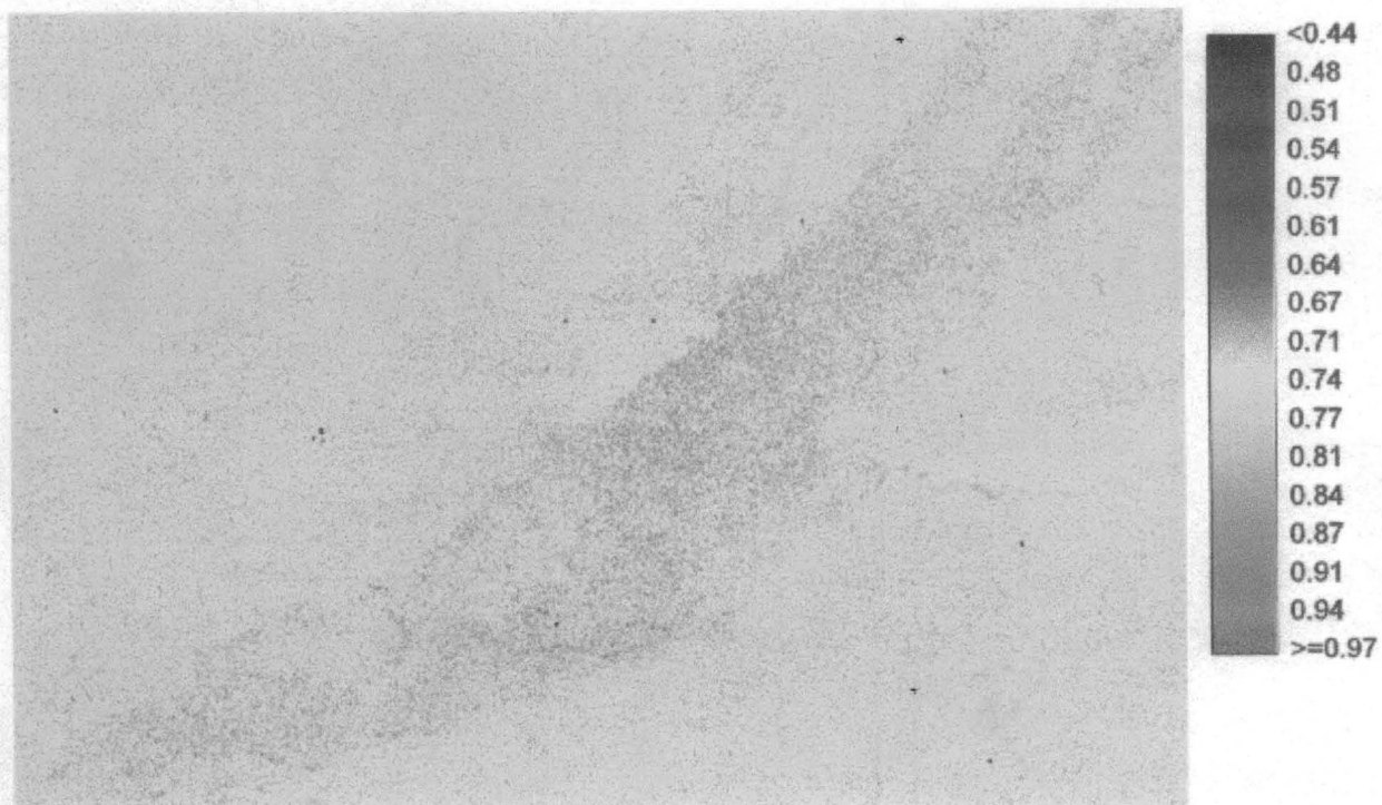
Fig 4.1 TTVI vegetation index image of the study area using bands 2,3 of MSS(1976)
