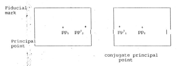
Fig 5 shows relative points of fiducial and principal point for adjacent photographs
