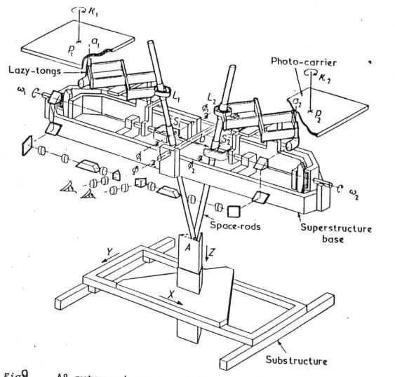
Fig9 A8 autograph space-rod diagram. (Wild, Heerbrugg Ltd of Switzerland).
