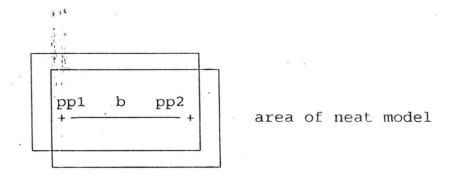
Fig 6 shows sketch of area covered by one model. The distance between any adjacent principal points pp1pp2 is the
