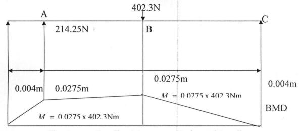
Fig. 5: Bending Moment at Horizontal Loading
