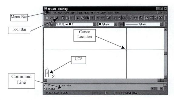
Figure 2.6 AutoCAD DRAWING EDITOR
