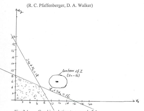
Fig. 3.1 Graphic solution to example 3.1
