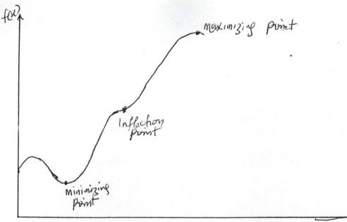
Fig. 1.4 Possible Solution Points to  $df(x)/dx_j=0$
