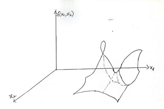
Fig. 1.5 Two Dimensional Saddle Point
