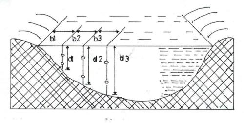
Fig. 1.6.1 <u>View of a stream cross-section showing location</u> of points of observation.
