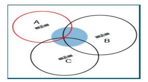
Fig.2.1: GPS Trilateration Illustration (Source: I.O.P, 2014).
