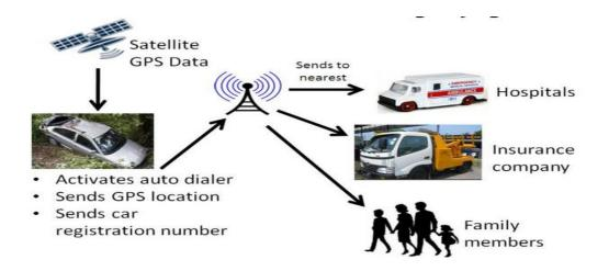
Fig.1.1 Automatic Accident Location Detection System (AALDS) (Goh *et al.*, 2014)
