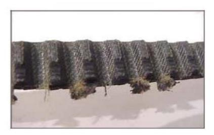
Plate VII: excessive edges wear (Gates, 2010)
