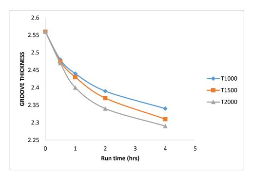
Figure 4.3: Variation of belt groove thickness with run time
