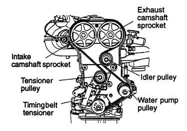
Plate XIX: Engine timing system parts identification (Auto, 2017)
