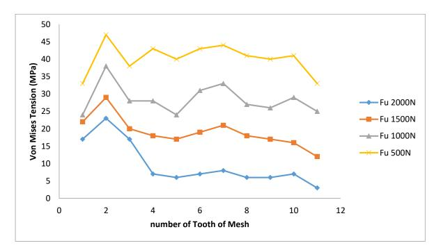
Figure 4.9: Load distribution on teeth in mesh due to the pre-tensioning force
