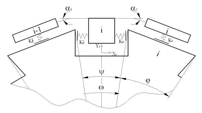
Plate XXIV: Basic model of the belt with belt pulley (Gerbert, 2010)
