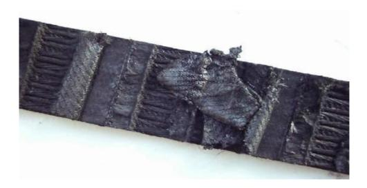
Plate XI: Melting from high temperature operation (Stojanovic, 2011)
