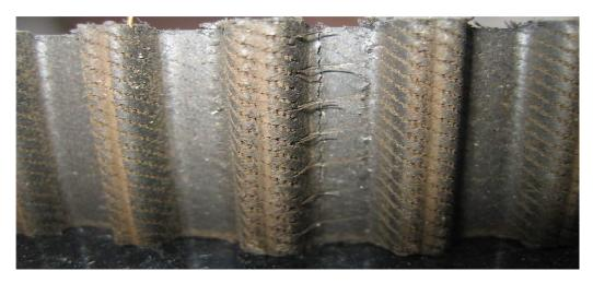
Plate IX: Damage of the face surface of the belt (www.researchgate.net/publication)
