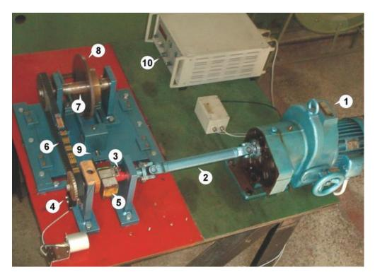
Plate XXI: Test bench for testing of timing belt
