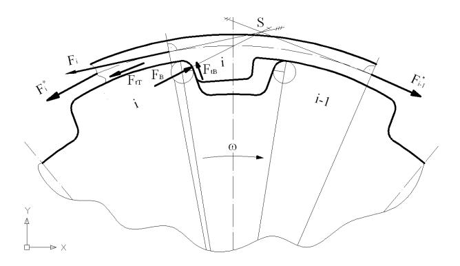
Plate XXIII: Forces and resistances on the belt and driving pulley due to meshing (Karolev, 1995)
