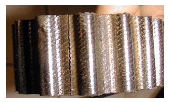
Plate V: Crack in the belt tooth root (www.researchgate.net/publication/271705831)
