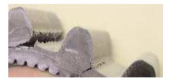
Plate VI: Shear in the belt tooth root (www.researchgate.net/publication/271705831)
