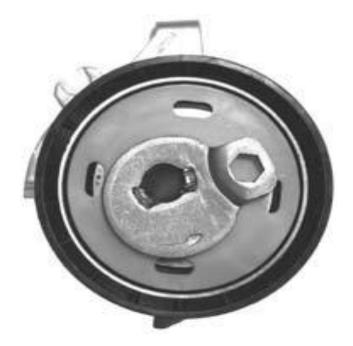
Figure XVI: Automatic Spring-Loaded Tensioner (Auto, 2017)
