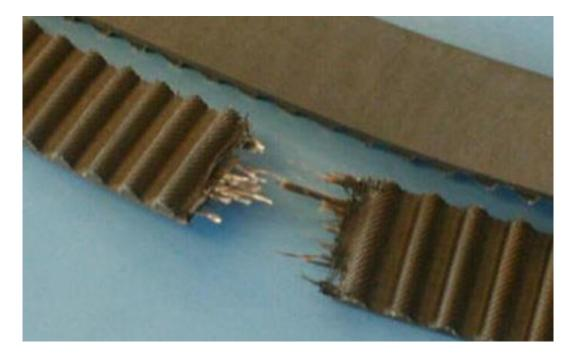
Plate II: Cracking of the drive element (www.researchgate.net/publication/271705831)
