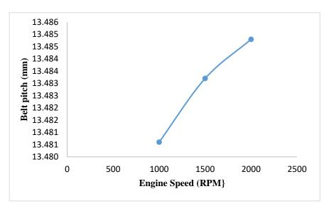
**Figure 4.2: Variation of belt Pitch with Engine speed**
