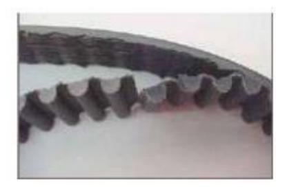
Plate X: Back crack (Stojanovic, 2011)
