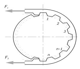
Figure XXII: Belt meshing with belt pulley (Stojanovic, 2009)
