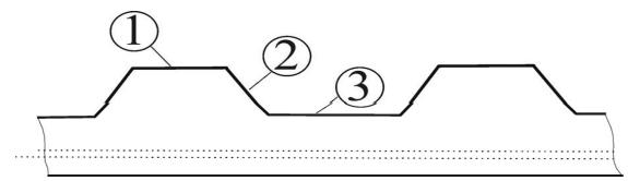
Figure 3.1: Measuring points on the belt for measurement of roughness parameters (B. Stojanovic *et al.*, 2009)
