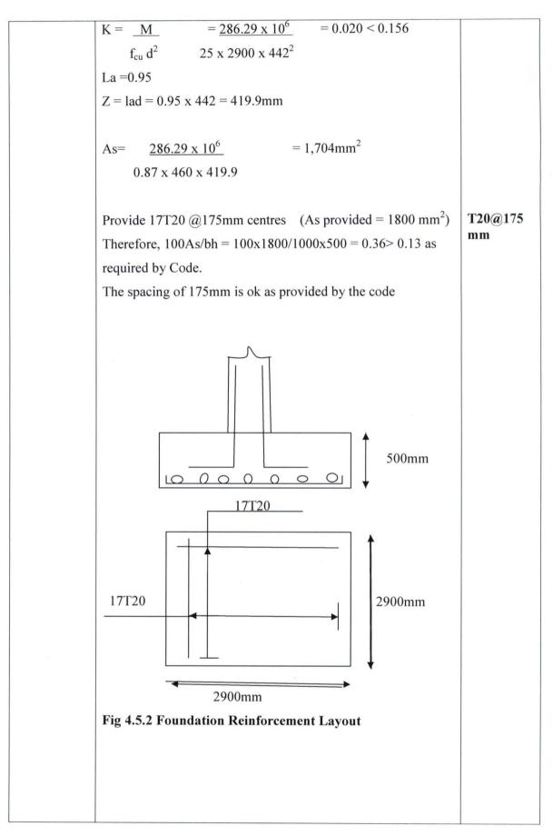
Effective depth = 500 - 40 - 8 = 452mm Net upward pressure = Earth pressure - self weight  $211.40 - (1.4 \times 24 \times 0.5) = 194.60$ kN/m<sup>2</sup>
