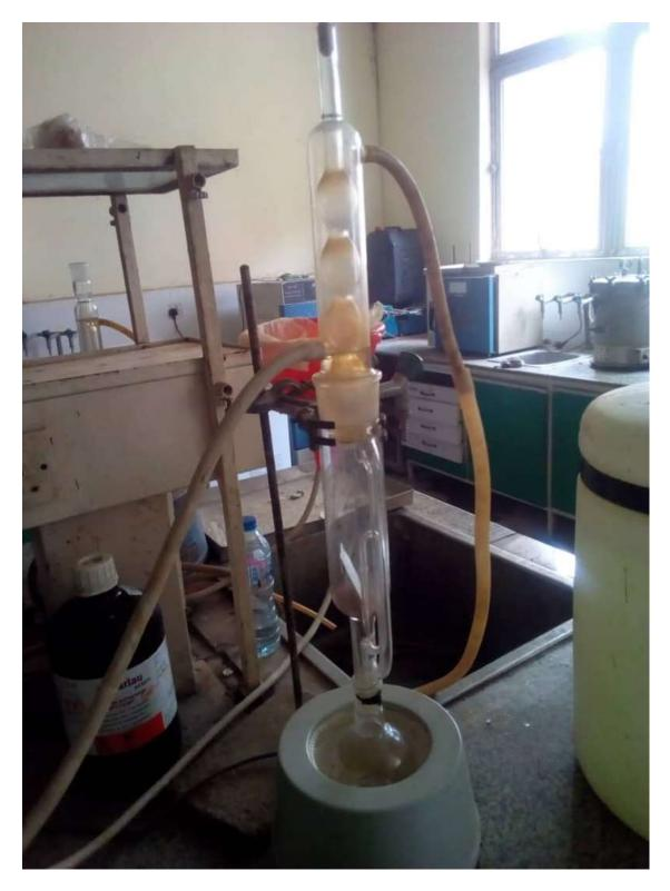
Figure 3.2d. Soxhlet apparatus for the separation of maltene and asphaltene fractions from bitumen
