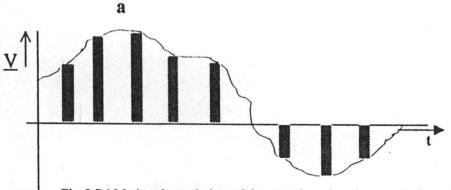
Fig 5 PAM signal consisting of the samples of analogue telephone signal a
