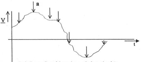
Periodic sampling of the analogue telephone signal a
