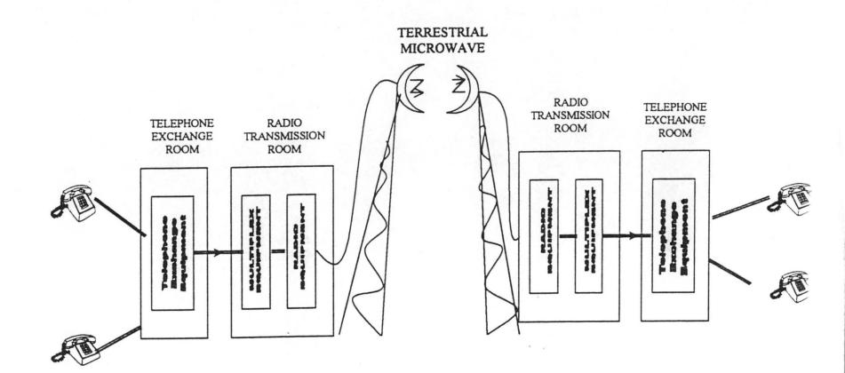
FIG 7 TRUNK CALL SEQUENCE AND THE MULTIPLEX
