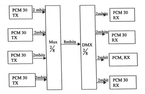
The output signals of 4 PCM 30 are combined to a signal of 8-bit/s and transmitted via a common transmission path to the receiving side (multiplex procedure).
