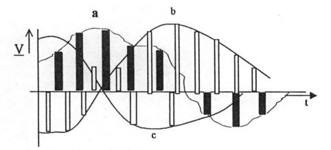
Fig 6 PAM signal consisting of the samples of analogue telephone signal a
