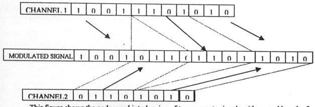
This figure shows the code word interleaving of two separate signals with a word length of four bits
