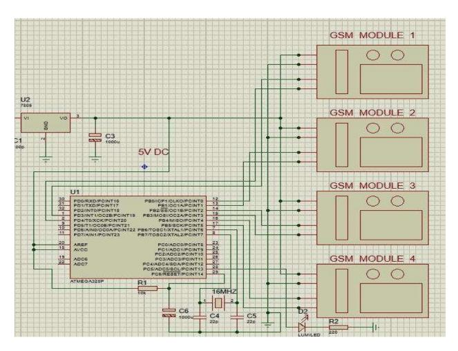
Figure 3.7: GSM Module Interfacing
