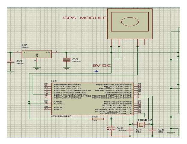
Figure 3.5: GPS Module Interfacing with MCU
