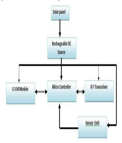
Figure 3.2: System block diagram of the master node
