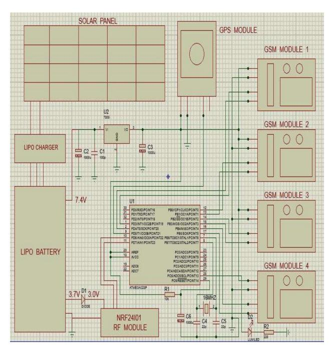
Figure 3.8: Master Node Circuit.
