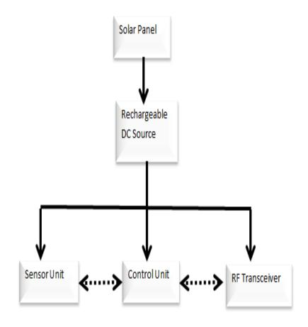
Figure 3.9: Block diagram of slave node
