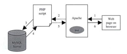
Fig 4.1 the step by step process of how MySQL, PHP and Apache work together.
