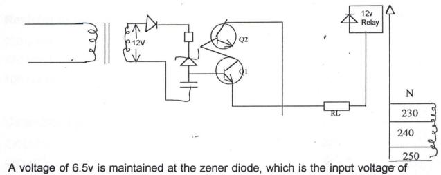
the transistor. The output voltage is calculated using direct-coupled amplifier method. For directly coupled amplifier, the output is twice the input voltage i.e.  $V_0 = 2Vi$ . So, since Vi = 6.5v therefore Vo = 2 x 6.5 = 13v. This stabilizer is designed to deliver 500w, so the current (I) will be power divided by voltage, which is equal to 2.08A (i.e. P/V = 500/240)
