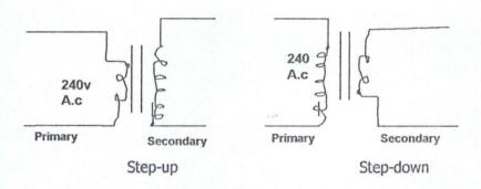
For this power supply the transformer used is a step down transformer since most modern electronic circuit operate at voltages well below 240v.
