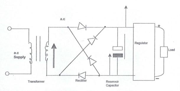
Block arrangement of a typical mains-operated d.c power supply.
