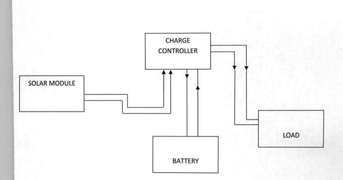
Fig.3.1: circuit diagram of the solar powered lighting system.
