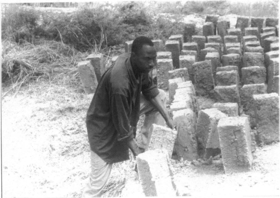
Plate 1: PICTURE SHOWING SOME SELECTED SAMPLES OF THE MOULDED SOILCRETE BLOCKS.
