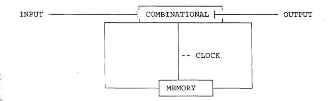
There are several methods of implementing flip-flops and each involves cross-coupled configuration to provide the feedback that creates latching effect. Most sequential circuits contain many flip-flops that are synchronised together by a master clock to provide no time intervals between clock pulses at the final states and to provide system timing to accomodate both short and long operations.
