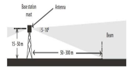
Figure 2. 2: Direction of coverage due to a Base Station Antenna Source: Adopted from (Mousa, 2011)
