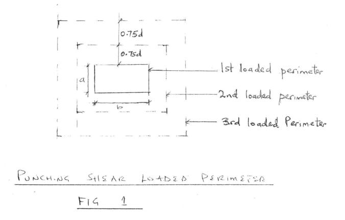
The max shear stress is calculated from Vmax = vp/[2(a + b)]dp and should not exceed 0.8 fcu or 5N/mm<sup>2</sup> whichever is the lesser.
