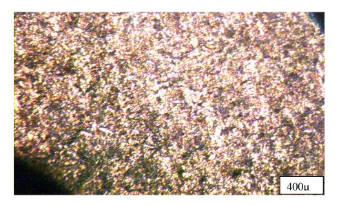
Plate 4.5 Micrograph of etched Aluminium test sample using Zungeru sand
