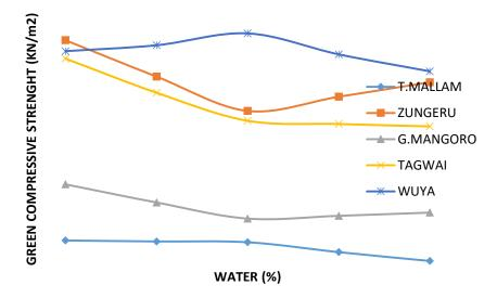
Figure 4.2: Variation of Green Compressive Strength with Water Content
