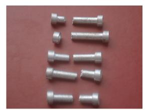
Plate 3.5: Alumiunm Cast Samples after Tensile Tests
