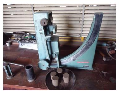
Plate 2.1: Ridsdale-Dietert Universal Sand Strength Machine, FIIRO Laboratory
