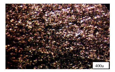
Plate 4.1 Micrograph of etched Aluminium test sample using Gidan Mangoro sand
