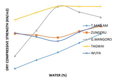
Figure 4.3: Variation of Dry Compressive Strength with Water Content
