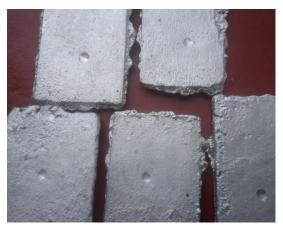
Plate 3.6: Aluminium Cast Samples Showing Indention of Hardness Tests
