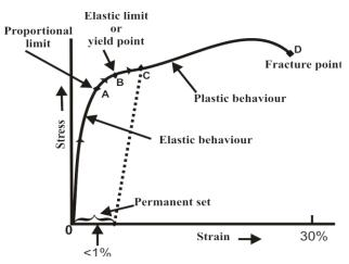
Figure 2.2: Stress-Strain Diagram of a Ductile Material (Hearn, 2000).
