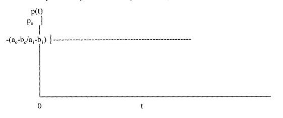
From the above diagram p(t) fluctuates about the value  $-(a_0-b_0/a_1-b_1)$  with period  $2\pi$
