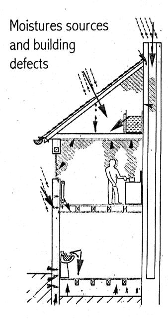
Fig 3.2 moisture sources and building defects
