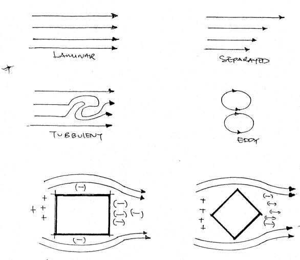
AIR FLOWING AROUND À BULLDING WILL CAUSE UNSVEN POSITIVE AND NEGATIVE PRESSORE AREAS TO DEVELOP.
