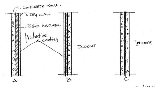
THE PLACEMENT OF MASS RELATIVE TO THE INSULATION.
