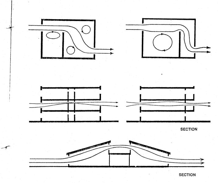
FIG 3.58 EXPLAINS THE DEPTH OF A ROOM WHICH HAVE EFFECT ON VENTILATION. OPEN PLANS MOST EXPECIALLY IN THE WARDS WHERE PATIENTS STAY, ARE PREFERABLE BECAUSE PARTITIONS INCREASE THE RESISTANCE TO AIR FLOW AND THEREBY DECREASE TOTAL VENTILATION
