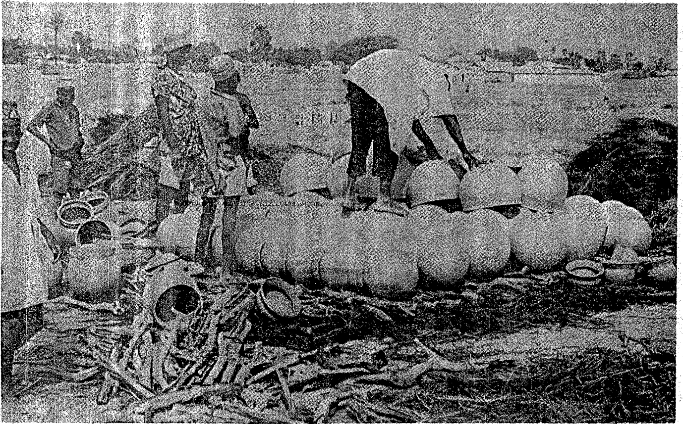
PLATE 3 Stacking the firing takes up to two hours. Stacking pots end to end allows efficient circulation of heat. 36)
