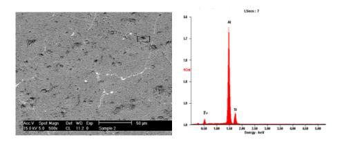
Plate VIII: SEM of the Aluminium Alloy Figure 4.2: EDS of Aluminium Alloy
