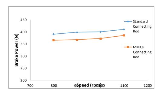
Figure 4.8: Variation of Brake force with Engine speed ratio
