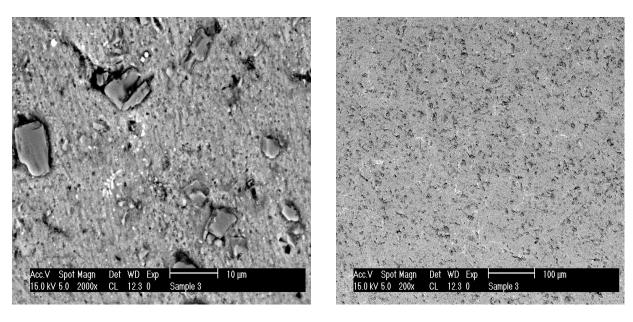
Plate X: SEM of the aluminium alloy with 6% by weight CSAp
