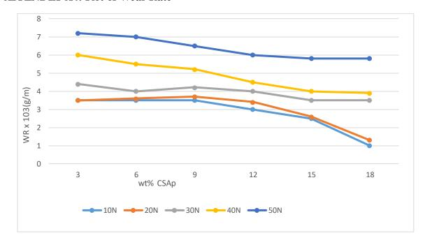
Figure A 4: Variation of wear rate with wt% of coconut shell ash particles
