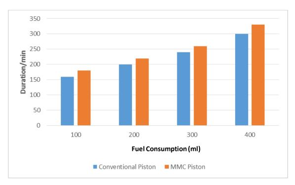
Figure 4.7: Performance Evaluation of Conventional and MMC Piston
