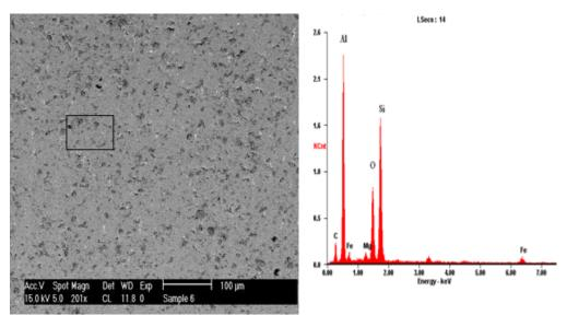
Figure 4.3: EDS of 3% by weight CSAp
