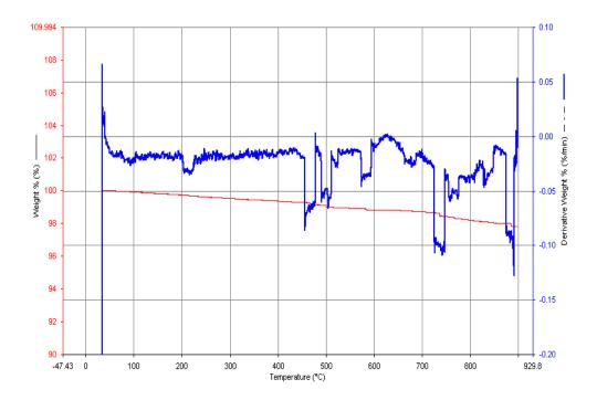
Figure 4.4: DTA/TGA of Al-Si-Fe Alloy
