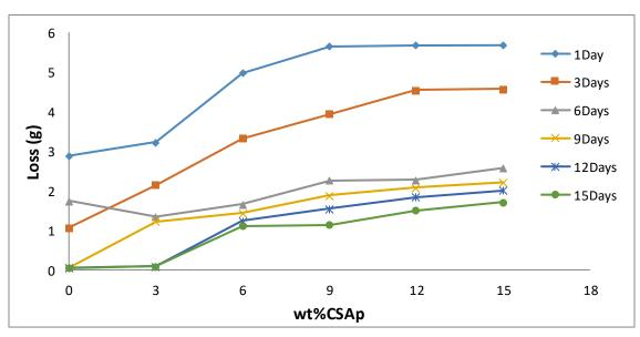
Figure: A6: Average Corrosion Rate Al-Si-Fe/Coconut Shell Ash (CSAp) Composites Immersed In 3.5%NaCl Solution
