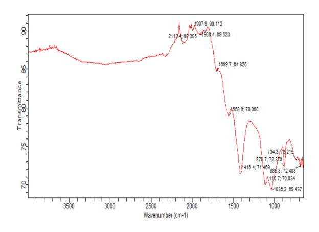
Figure 4.6 FTIR Spectrum of the Coconut Shell Ash
