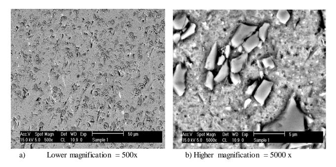
Plate XII: SEM of the aluminium alloy with 12% by weight CSAp
