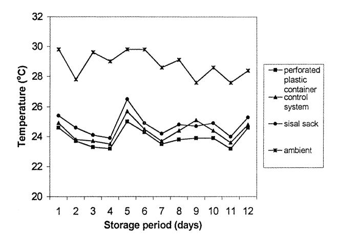
Figure 6: The effect of temperature on stored tomato inside the system.
