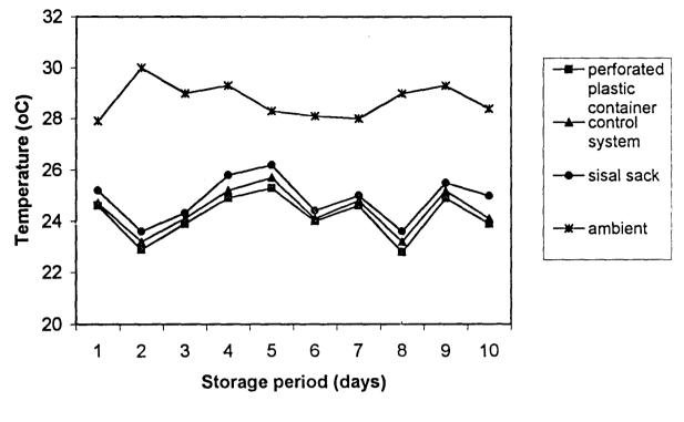
Figure 5: The effect of temperature on stored garden egg inside the system.
