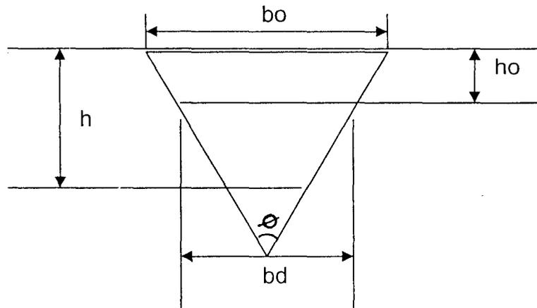
Fig. 1: Belt Drive Section
