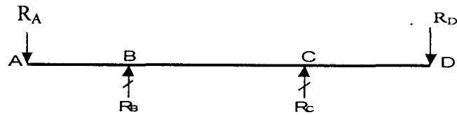
Fig7. Free body diagram of shaft of transmission unit
