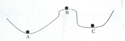
Fig 1.2: Stable and Unstable equilibrium of a ball on a hill..
