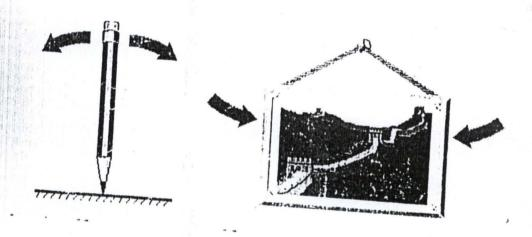
Fig 1.1: An Illustration of stable and unstable equilibrium of an object.
