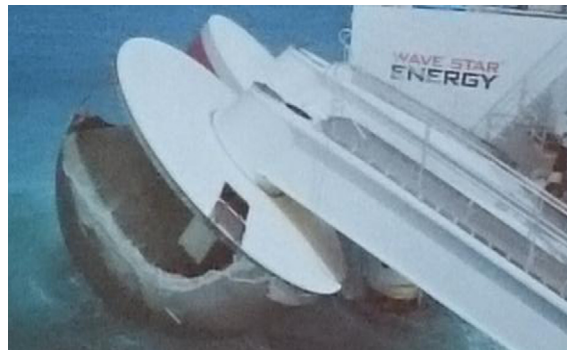
Fig. 9. A fractured buoy (courtesy of Wave Star Energy).
