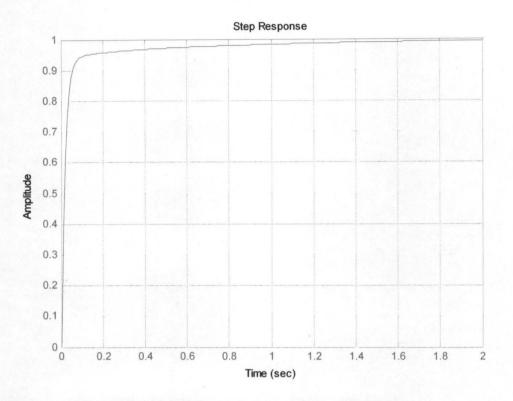
FIG. 3.9 CLOSED – LOOP STEP:  $K_p = 350K_I = 5500$
