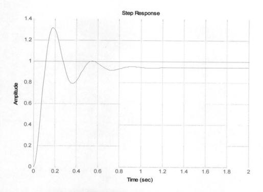
FIG. 3.7 CLOSED – LOOP STEP  $K_p = 300, K_d = 10$
