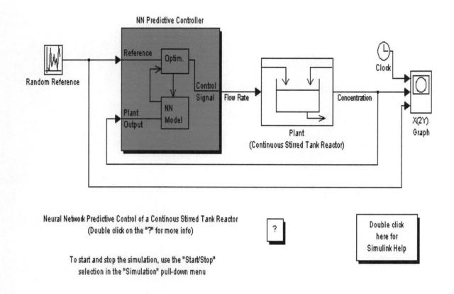
The continuous stirred reactor tank has the following embedded dynamic transfer diagram
