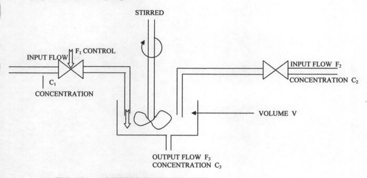
FIG. 1.3 STIRRED TANK REACTOR
