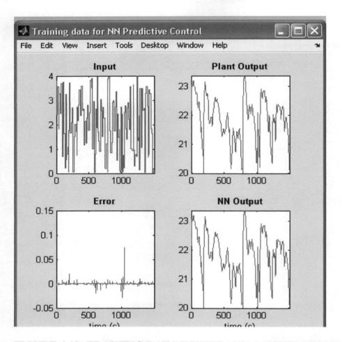
FIGURE 4.13: TRAINING DATA INPUTS AND OUTPUT PLANT, ERROR AND NN OUTPUT SIGNALS
