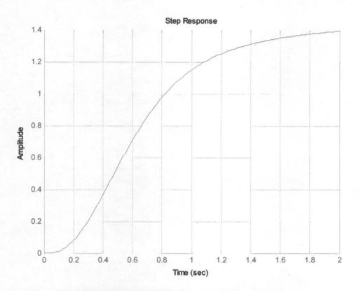
FIG. 3.8 CLOSED-LOOP STEP:  $K_p = 30 K_1 = 70$
